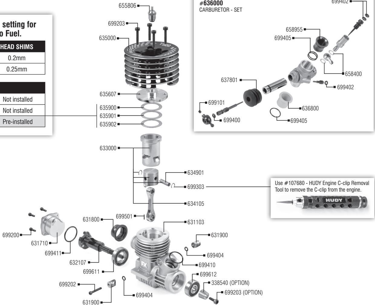
Use #107680 - HUDY Engine C-clip Removal Tool to remove the C-clip from the engine.
